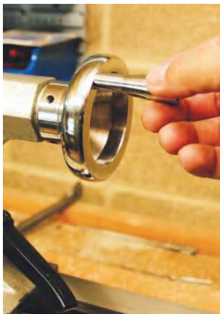
▲ Top quality fittings, such as the quill advance, are a theme throughout the lathe
